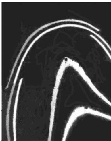
FIGURE 6.12. Multiple fringes of variable chromaticity meeting across a step. The lighter fringe corresponds to the red and the darker one to the green radiation as they appear in the original, which was in color. (From Shaalam and Little, 1975.)
