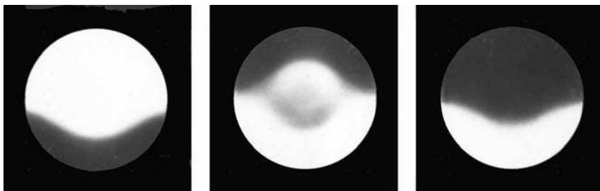
FIGURE 8.13. Foucault graphs of an aspherical mirror.
