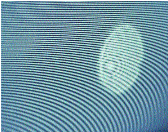
Figure 3. Fringes on test surface
